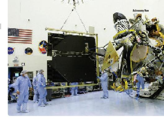
even months after its August 2005 launch, NASA's Mars Reconnaissance Orbiter(MRO) will surf its way into orbit around Mars. At a hefty 2,180 kilograms, the spacecraft is no lightweight and is the first spacecraft designed from the ground up for aerobraking – using the atmospheric drag of a planet to slow down a spacecraft, modifying the probe's orbit. Get it wrong and the spacecraft will burn up as it plunges to the surface of the planet.
